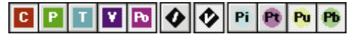
Figure 6: The 11 Show buttons control the types of symbols the ObjectBrowser will display. From left to right, they are: Constants, Procedures or Functions, Types, Variables, Properties, Inherited, Virtual, Private, Protected, Public, and Published.
